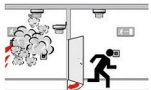
End evacuation, transfer of personnel and Cut off the door holder power supply, close the door.
